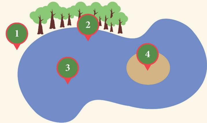
**3** Should be mostly bowl-shaped. Deep water up to 10 feet with a 1:3 slope should cover up to 75%; shallow water < 5 feet with a 1:10 slope should cover 25%.
